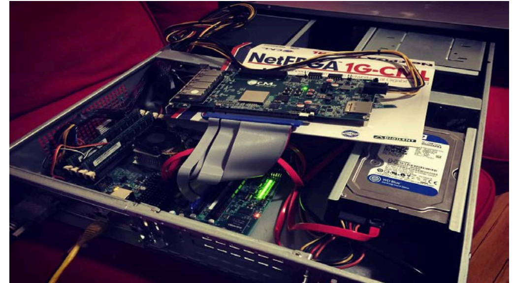
'Trilby': DMA Engine driven FPGA based workload accelerator built by Jon Masters for research into the barriers to adoption in the Enterprise, uses traditional approach of kernel driver and Operating System hacks.
